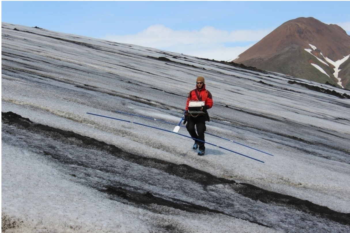
Ground-penetrating radar measurements on Múlajökull outlet glacier. Photo by Kristaps Lamsters.
